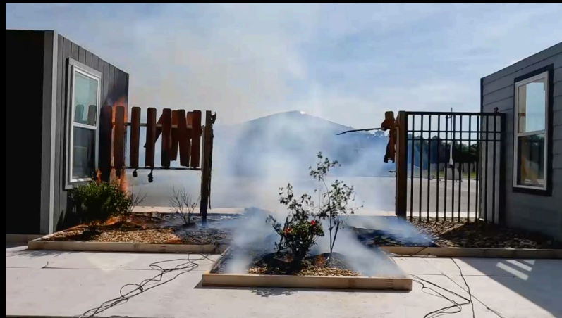
Ignition path via wooden fence
